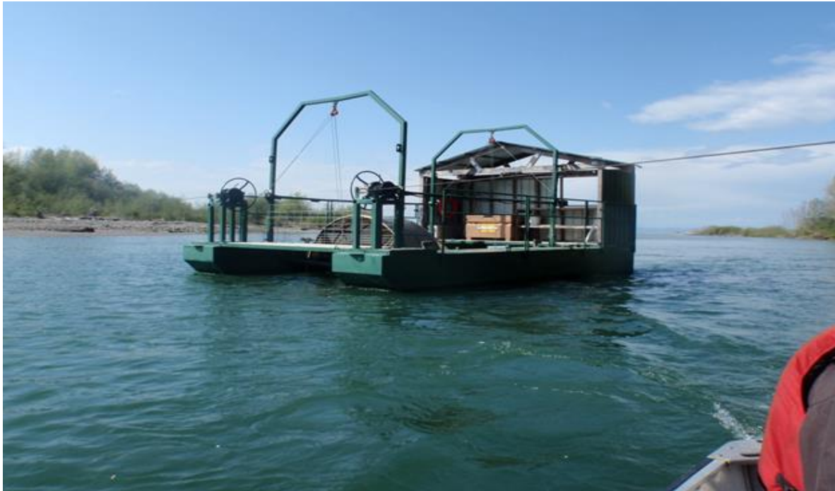
Figure 1. Top Elwha River 8' rotary screw trap fishing at Rkm 0.3 during the pre-project periods and bottom 5' rotary screw trap used during the dam removal period.
